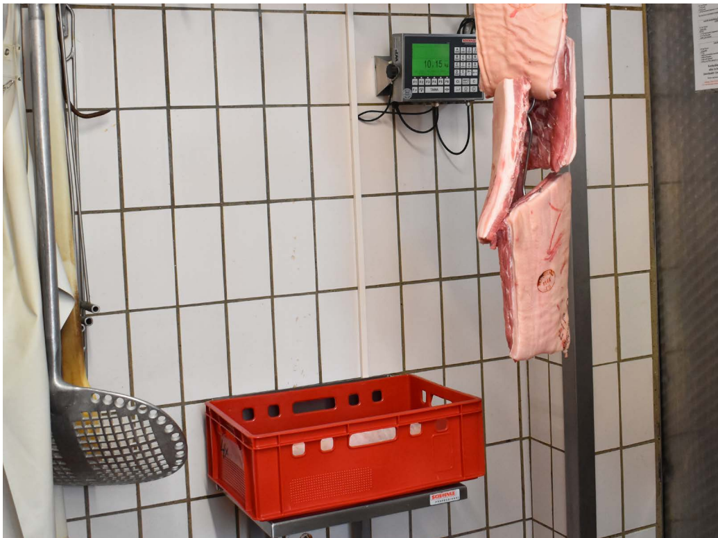
Overhead track scale and wall-mounted scale for fast, reliable weighing and control in the production flow
