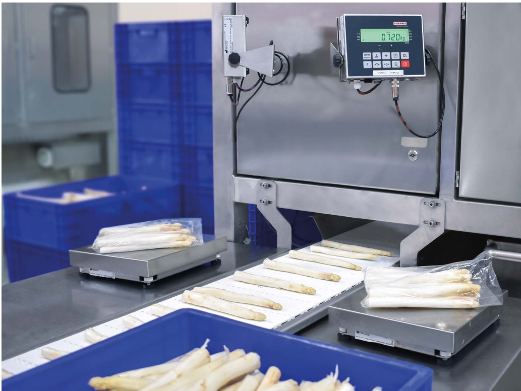
Stainless steel weighing platforms with terminal 3010 for fast and exact weighing on the assembly line
