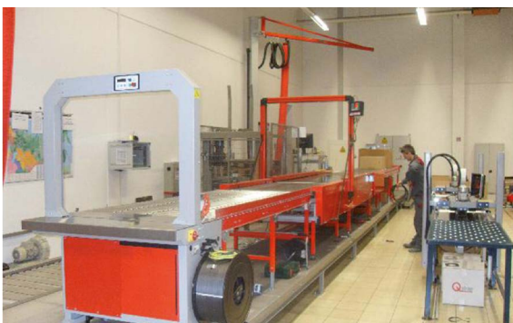
Parcel weighing with volume measurement
