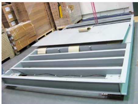
Heavy-duty scale with opened plate
