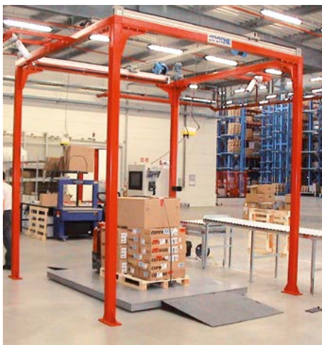
Volume portal, floor scale and drive-on ramp
