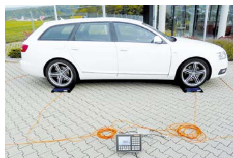
Wheel and axle load scale
