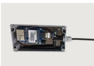
WLAN box for connection to serial interface, with economical power consumption optimal also for battery-powered systems.
