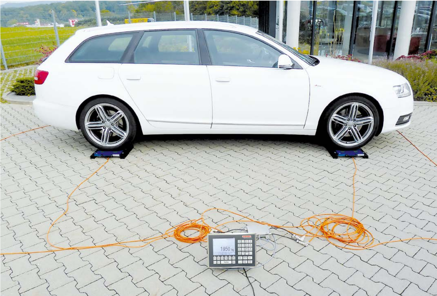
Example: 4 load plates can be interconnected into an overall weight scale
