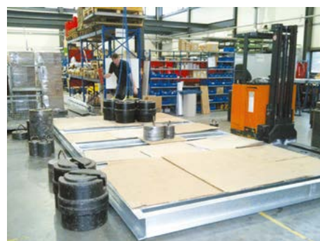
Floor scale calibration
