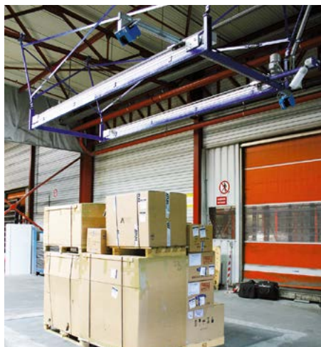
Ceiling module / volume, floor scale installed
