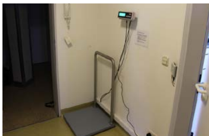
Three sides passable overground floor scale
