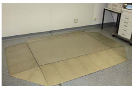
Three sides passable overground floor scale
