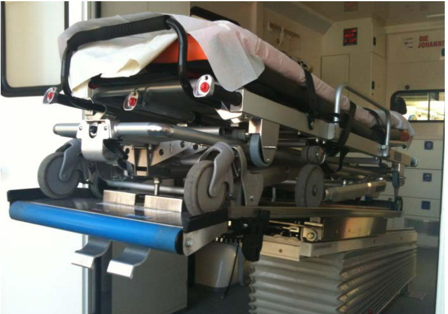
▶ A weighing system integrated into the stretcher rack can save lives in an emergency by improving the preclinical weight-adapted dosage of medicine
