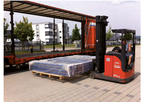
Load placement onto heavy-duty scale with special-purpose transport
