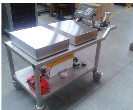
Double scale on mobile frame with rollers, barcode scanner and battery power
