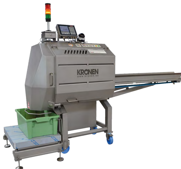
Vegetable slicer with dosing scale
